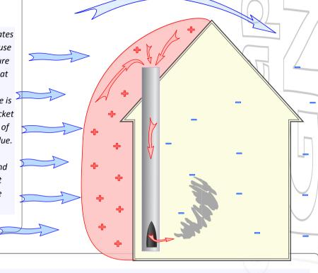
As an immediate solution, try to open a window slightly in the same room where the fireplace is. This should equalize inside and outside pressure giving your flue a chance to establish normal operation. However, this window test will significantly decrease efficiency of your fireplace because cold outside air will rush through the window.
